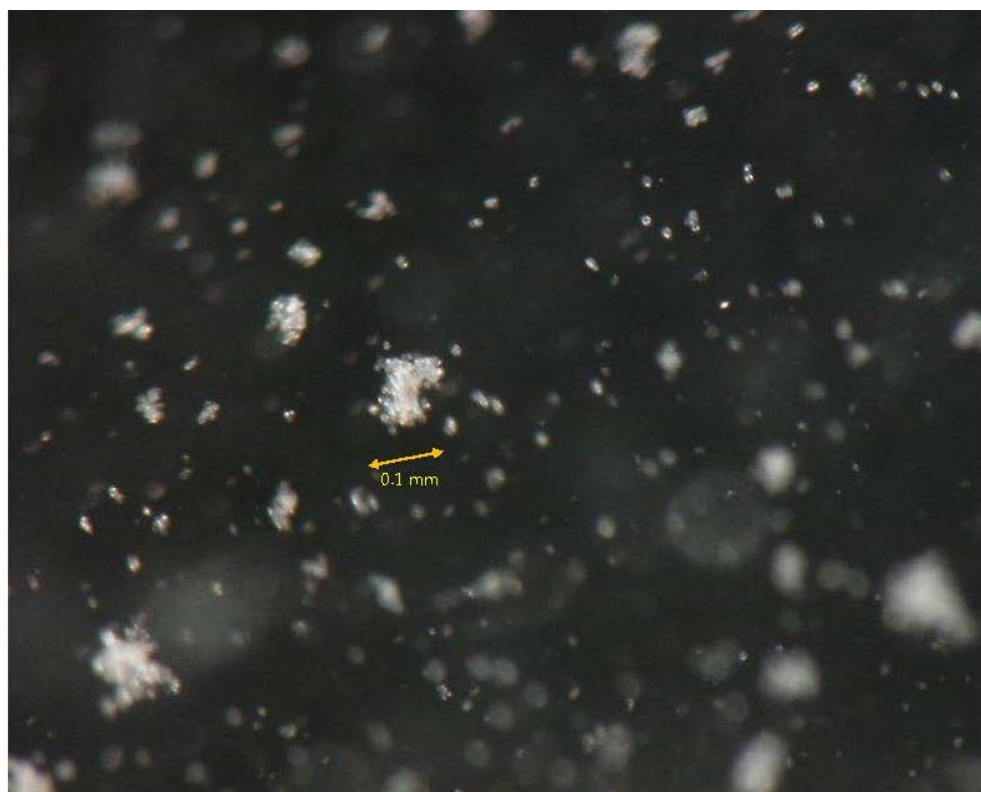
Figure 11. Digital image of aggregation, adsorption, and crystalline in the MICP process.
