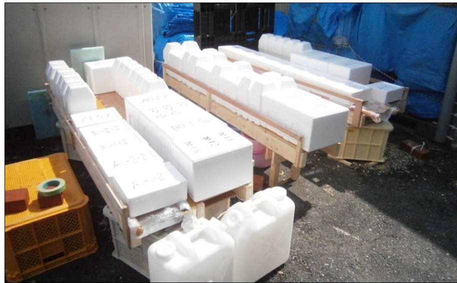
Figure 6. Curing setup of MICP experiments.
