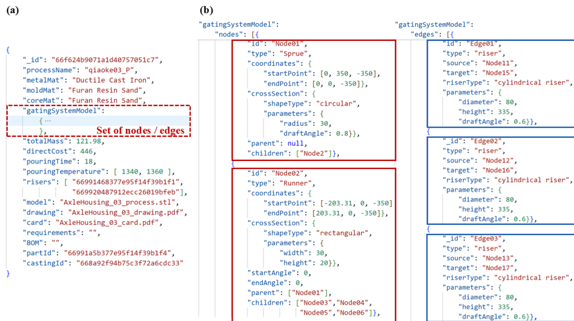
Figure 14. (a) The storage contents of the process data unit; (b) the specific parametric model information of the gating system. Red boxes represent nodes, and blue boxes represent edges, respectively.
