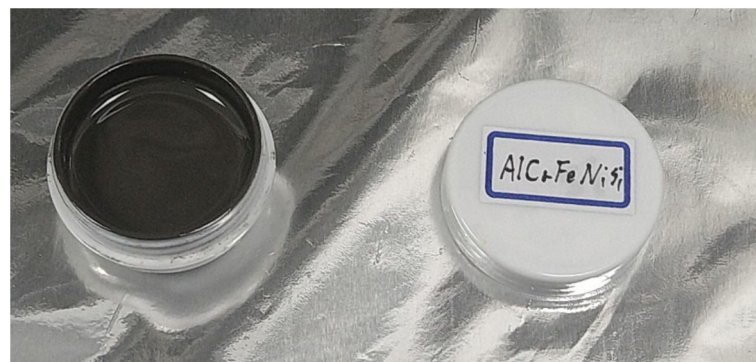
Figure 1. Mixing slurry with 60 vol.% HEA powder.
