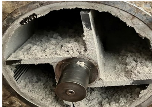
Figure 2. Fiber pulping using a cylindrical laboratory refiner.
