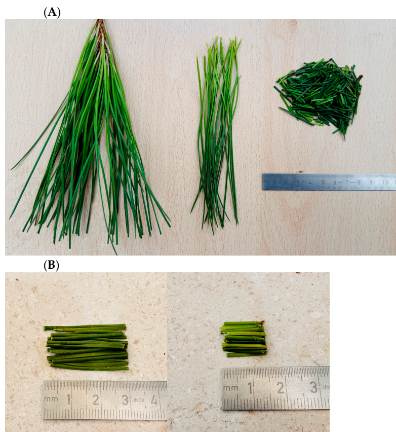
Figure 1. (A) Pine needles PN (left) as received, (middle) arranged in similar lengths, and (right) cut to 15 to 30 mm lengths and mixed. (B) Pine needles PN cut in different lengths of (left) 30 mm and (right) 15 mm.
