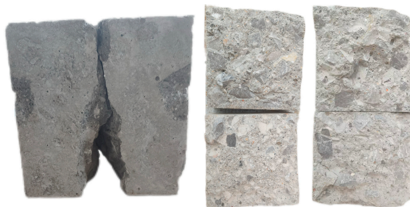
Figure 10. Forms of failure in cube splitting tensile strength test (150 mm × 150 mm × 150 mm).
