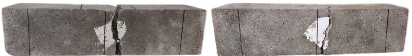
Figure 6. Forms of failure in flexural tensile strength test (100 mm × 100 mm × 400 mm).
