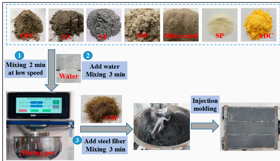
Figure 2. UHPC mixing process employed in this study.
