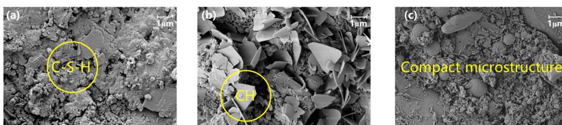
Figure 8. SEM microscopic morphology of the optimal group at different ages: (a) 3 h, (b) 1 day and (c) 28 days.
