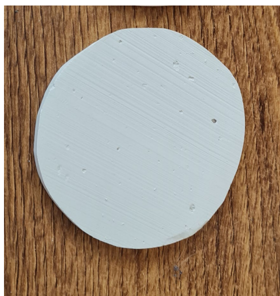
Figure 2. Photo of dry sample during preparation process. Surface irregularities, as well as shape and dimensions, are to be corrected using fine-gritted sandpaper.
