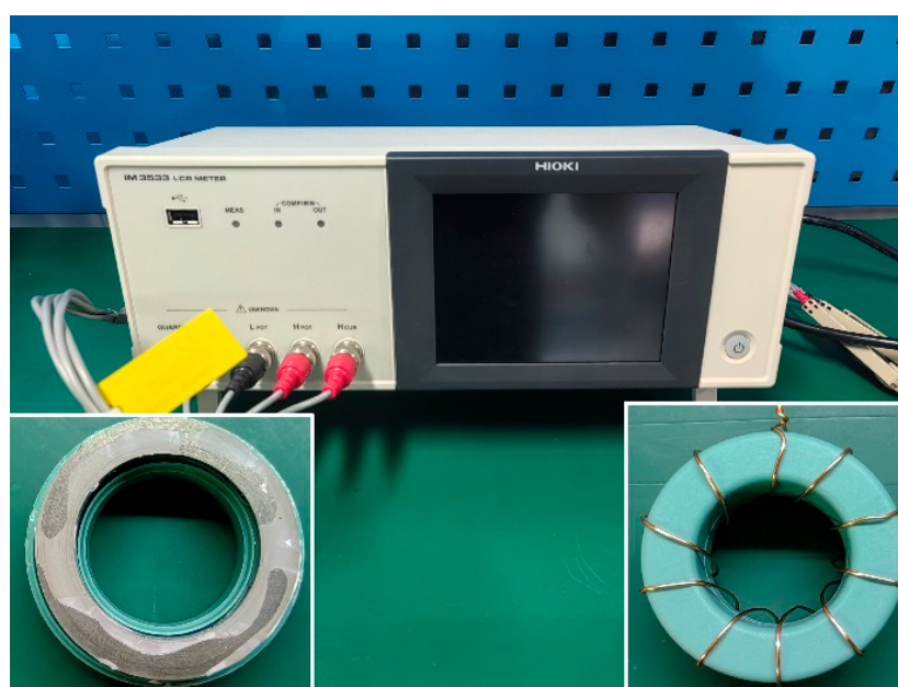
Figure 1. The IM 3533 LCR meter and Fe-based nanocrystalline magnetic ring.
