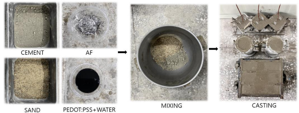
Figure 4. The test-sample production process.
