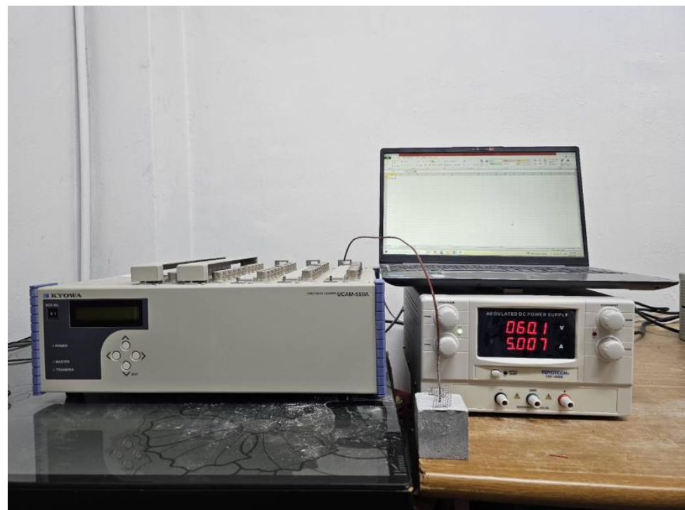
Figure 5. Thermal performance test setup.
