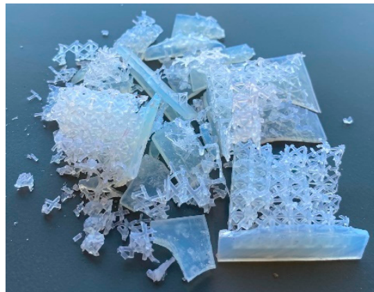
Figure 11. Shattered specimen after Charpy test.
