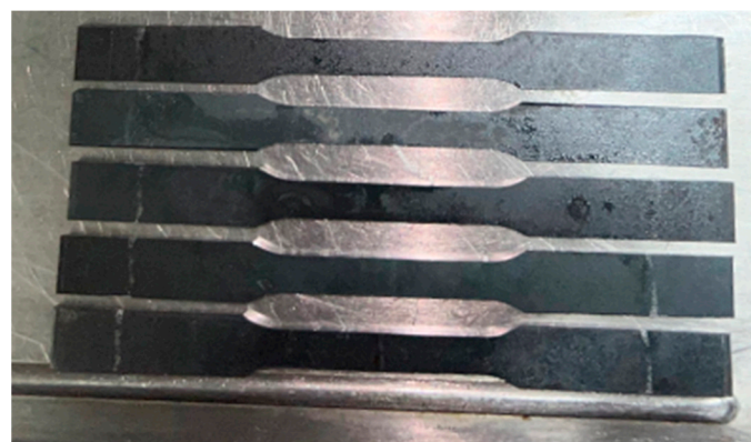
Figure 3. Specimens prepared for the static tensile test.
