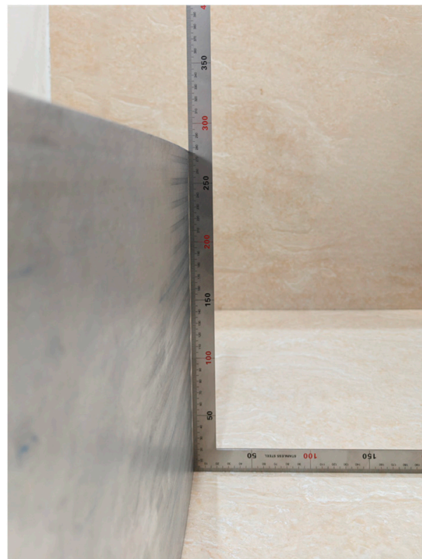
Figure 18. Generatrix straightness measurement method.
