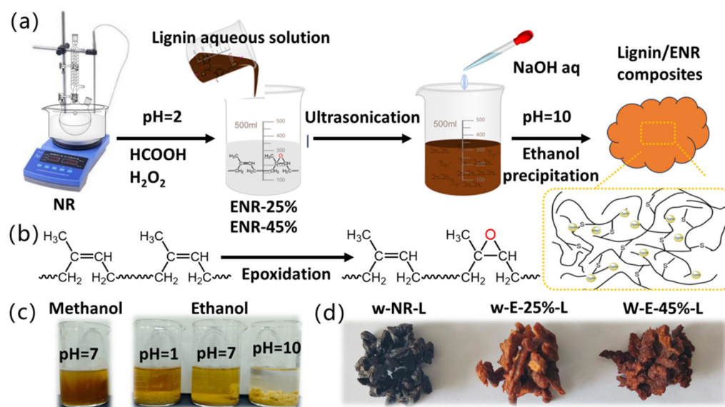
Figure 1. (a) Schematic diagram of wet mixing preparation of ENR/lignin compounds. (b) Epoxidation of natural rubber. (c) Precipitation of ENR/lignin compounds under different conditions. (d) Photos of ENR/lignin compounds with varying degrees of epoxy content.
