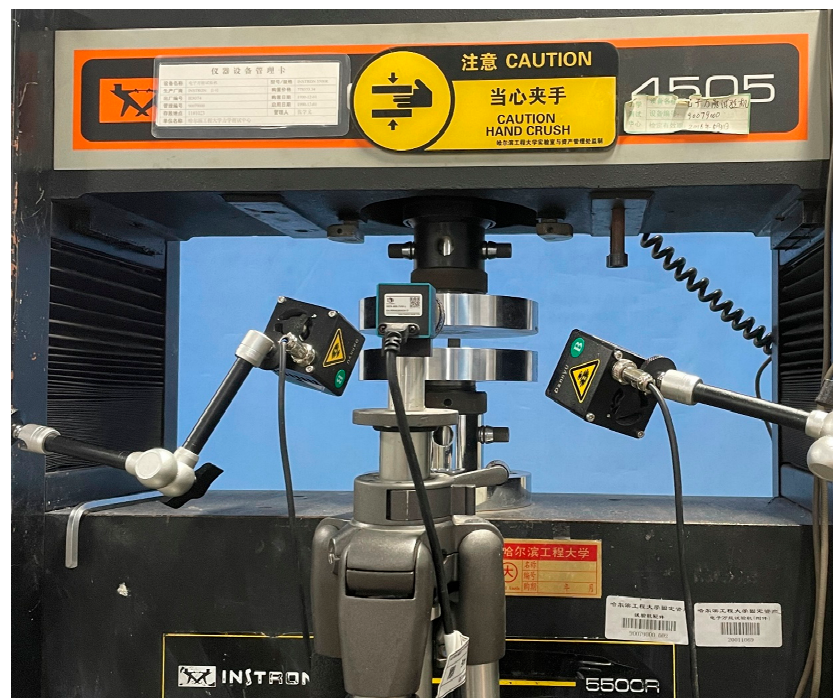
Figure 8. Picture of basalt-fiber laminate compression test.
