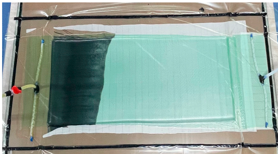
Figure 1. Preparation diagram of basalt-fiber laminates.
