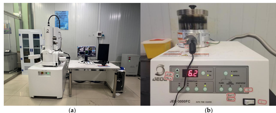
Figure 4. Scanning electron microscopy (SEM) testing equipment: (a) JEOL-JSM-IT800 thermal field emission scanning electron microscope; (b) JEC-300FC ion sputtering device.
