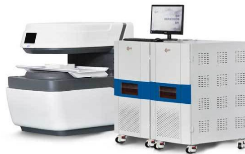
Figure 5. Low-field nuclear magnetic resonance measurement instrument, MacroMR12-150H-I.
