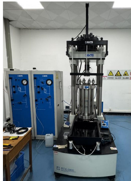
Figure 10. RTX-2000kN high-temperature and high-pressure electrohydraulic servo rock triaxial testing machine.
