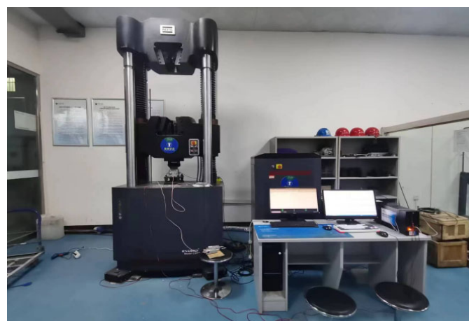
Figure 3. A 2000 kN microcomputer-controlled electro-hydraulic servo universal testing machine.
