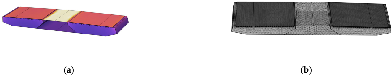
Figure 6. Configuration of bridge segment model. (a) Thermal field simulation diagram; (b) Grid division diagram.
