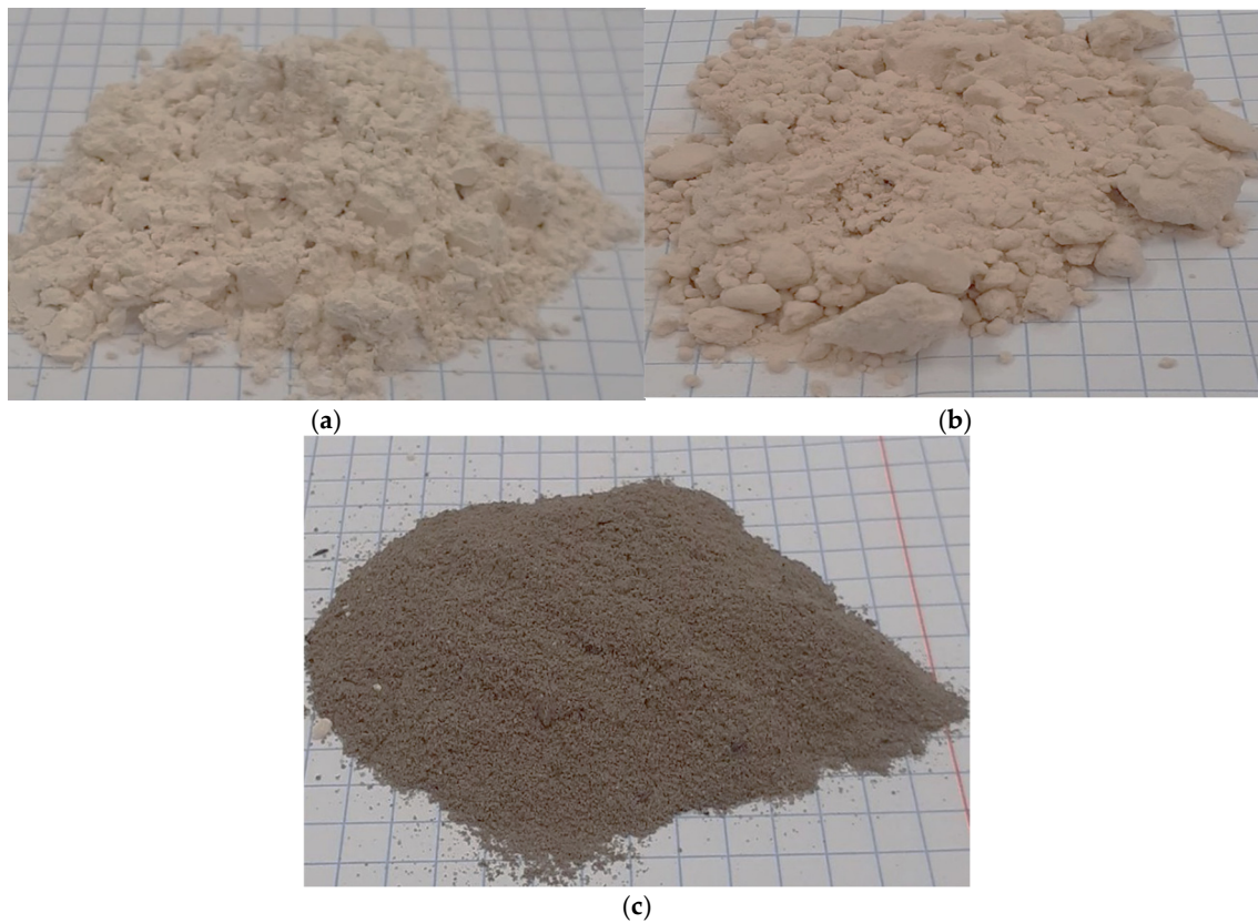
Figure 2. The waste materials used during the study: (a) ECO-ZEC, (b) PPR, and (c) fly ash.
