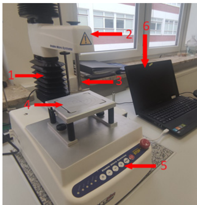
Figure 4. Station for determining crushing strength of granules [own study]: (1) overhead crane, (2) load cell, (3) measuring tip, (4) measuring platform, (5) controller with switch, and (6) computer with Exponent 6.1.27.0 software.
