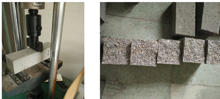
Figure 2. Post-failure specimens of the concrete samples.
