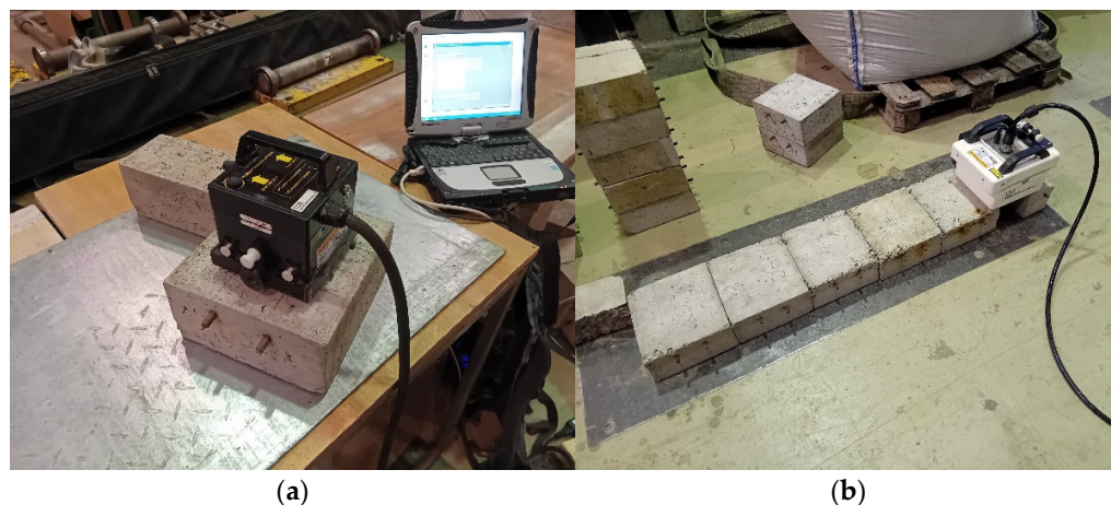
Figure 6. Scanning of concrete samples using GPR: (a) 2 GHz antenna, (b) 900 MHz antenna.
