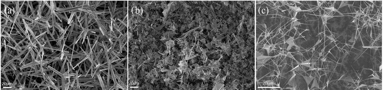
**Figure 1.** SEM images of different precursor particles: (a) tZnO powder, (b) sail-structured powder (c) sail-structured powder.
