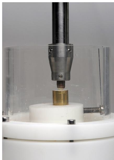
**Figure 2.** Sample positioned in a chamber of the chewing simulator. The sample is embedded in the metal sleeve, and the steatite sphere is positioned on the sample as an antagonist.
