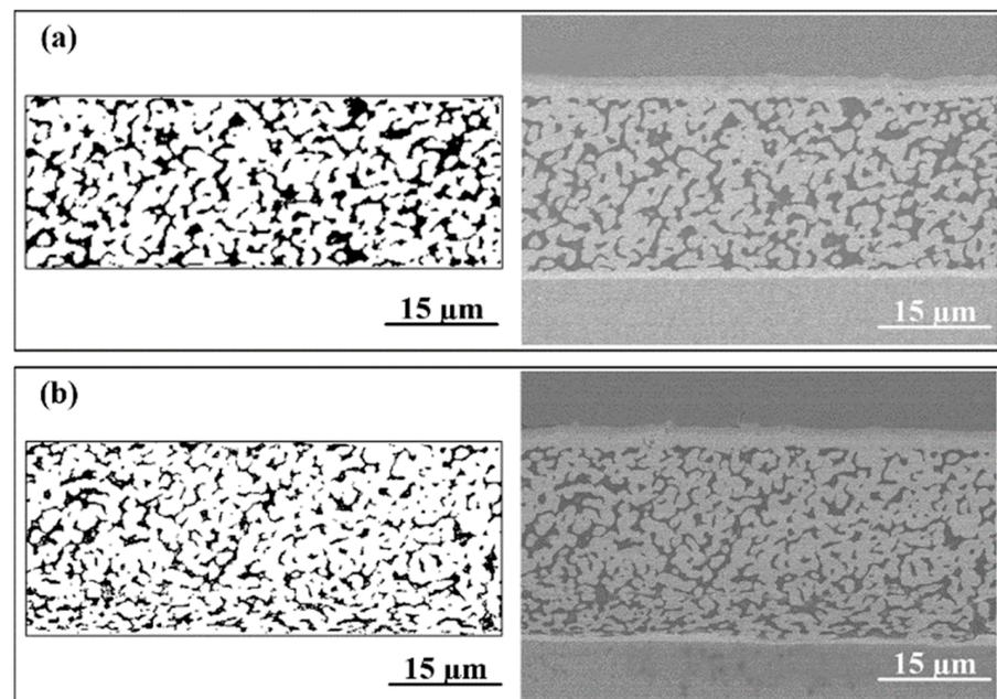
Figure 7. Microstructure of Ag-Au joints on different substrates after 100 h hydrothermal aging: (a) Au substrate and (b) Au-350 substrate.
