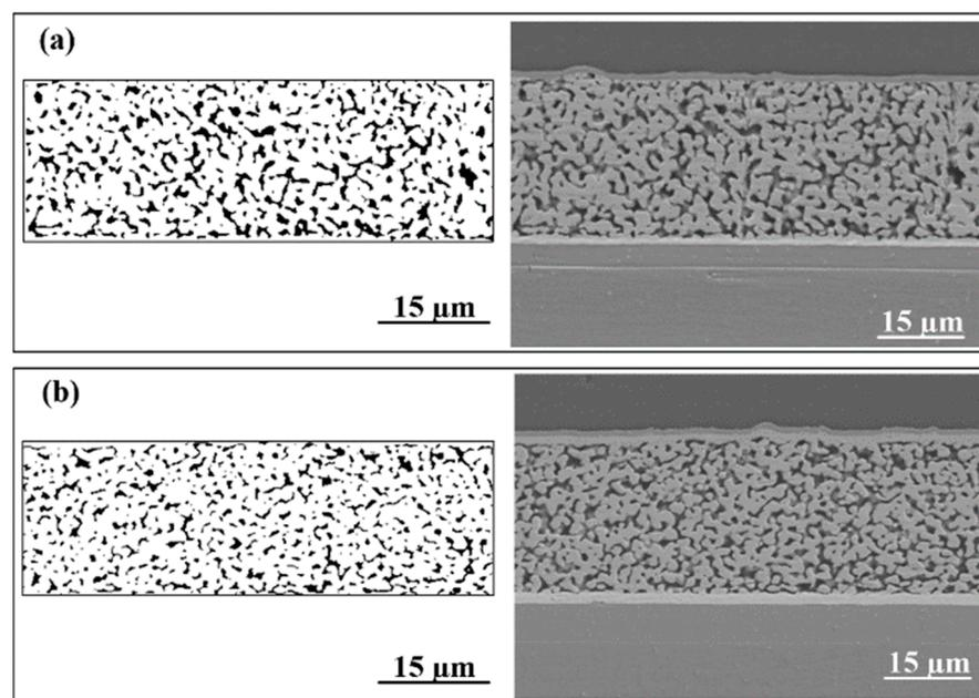
Figure 4. Microstructure of Ag-Au joints on different substrates after 200 h high temperature aging: (a) Au substrate and (b) Au-350 substrate.
