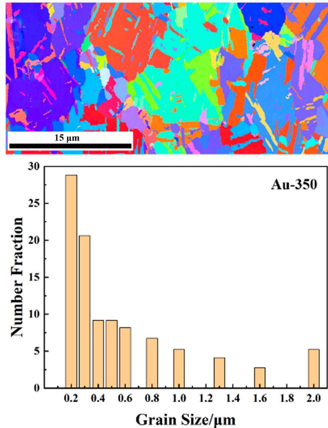
**Figure 2.** EBSD image and grain size distribution of the gold plating layer on the Au-350 substrate, grain orientation represented by different colors.
