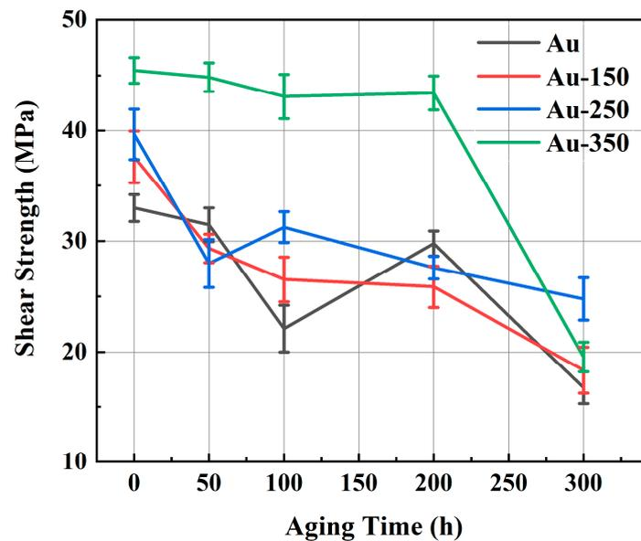
Figure 3. Shear strength of four kinds of Ag-Au joints with high-temperature aging.
