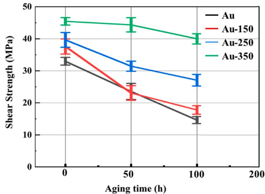
Figure 6. Shear strength of four kinds of Ag-Au joints with hydrothermal aging.
