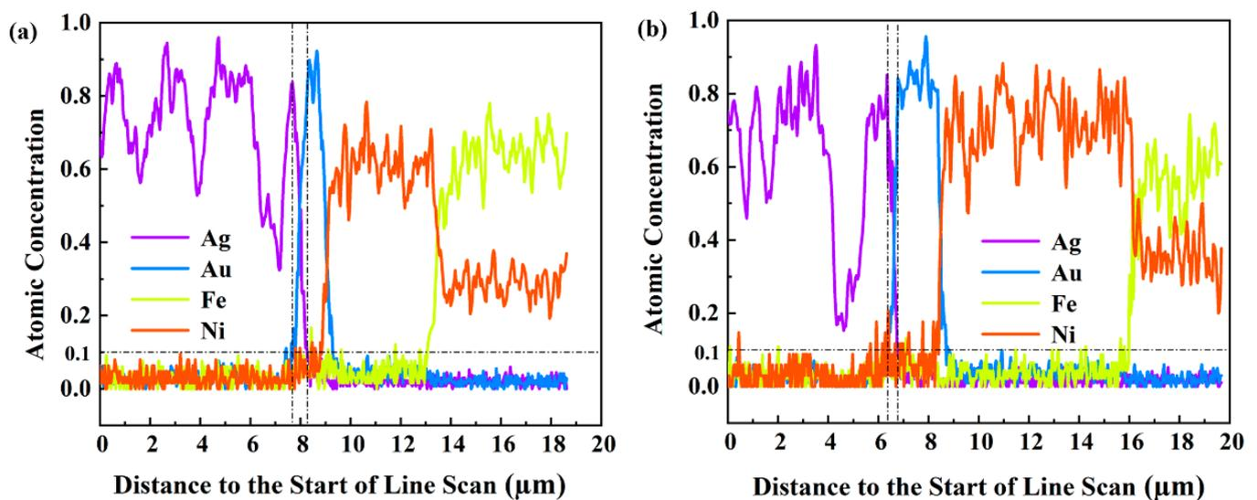
**Figure 5.** Diffusion zones of the joint interface between sintered Ag-Au joints on different substrates after 200 h high-temperature aging: (a) Au substrate and (b) Au-350 substrate.
