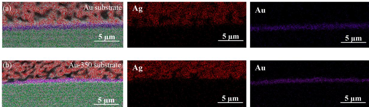
**Figure 8.** EDS area scan analysis of sintered Ag-Au joints on electrolytic Au under different preheated states after 100 h hydrothermal aging: (a) Au substrate and (b) Au-350 substrate. Red represents the silver element, purple represents the gold element.
