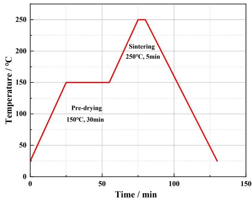
Figure 1. Sintering process.
