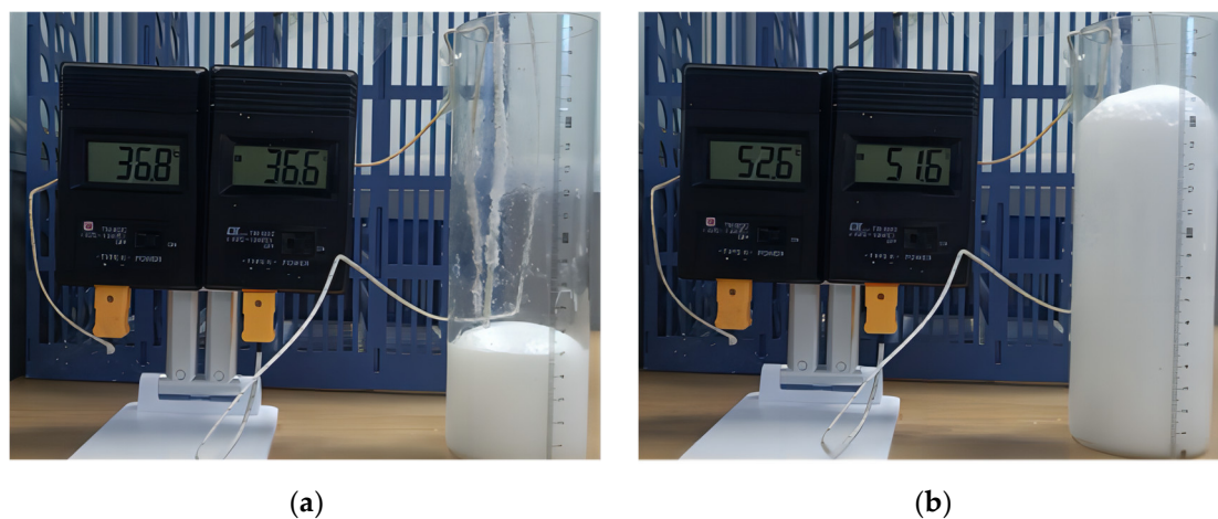
Figure 3. Volume and temperature measurement during grout expansion: (a) t = 14 s; (b) t = 28 s.
