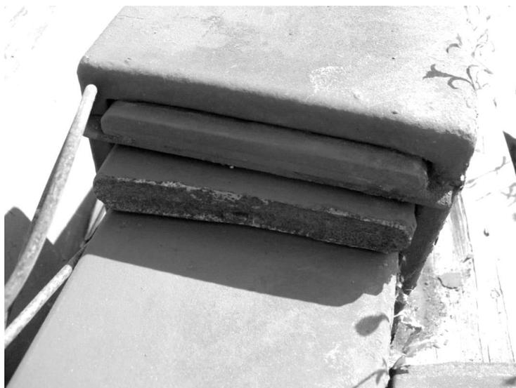
**Figure 1.** Fatigue fracture of the master spring leaf of a parabolic leaf spring.
