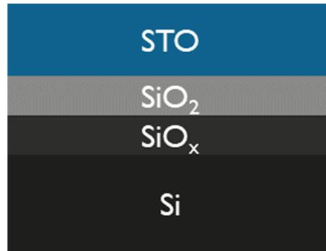
**Figure A1.** Layer stack used in ellipsometry fitting model.
