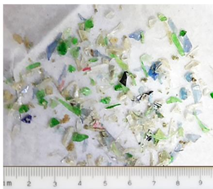
**Figure 1.** Sample of the PET microplastic.
