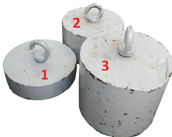
Figure 13. View of the prepared weights with the following masses: 1—10 kg, 2—20 kg, 3—30 kg [11].
