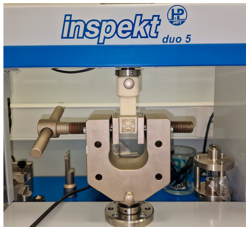
Figure 6. Lateral compression test on Universal testing machine Inspekt table 50 kN.
