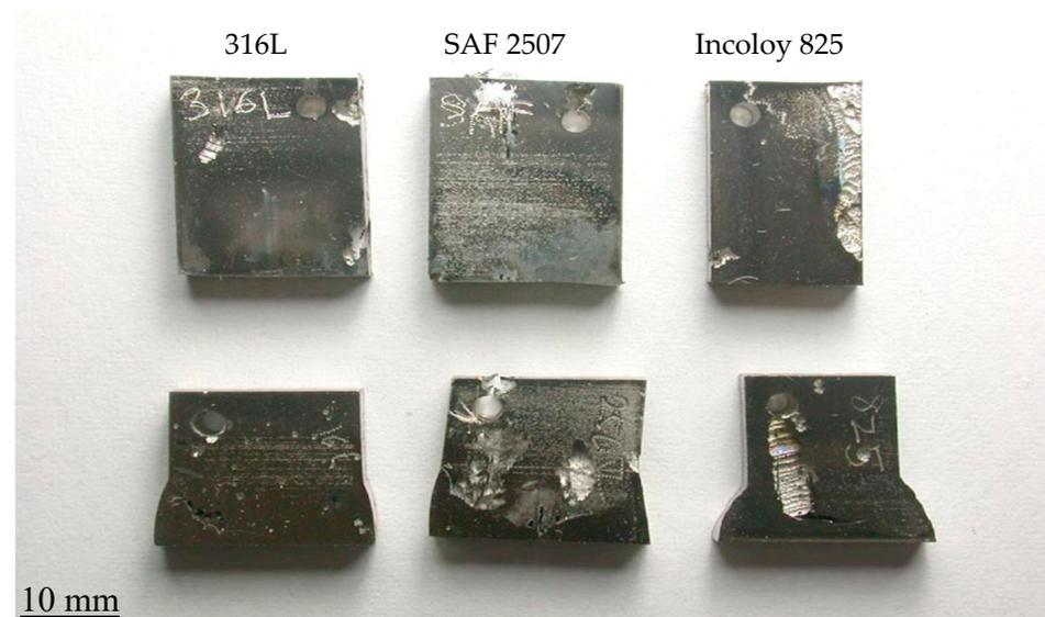
**Figure 8.** Appearance of coupons of parent metals and weldments of SAF 2507 and Incoloy 825 and 316L after exposure to a 6%  $\text{FeCl}_3$  solution (with no nitrite) at 50 °C for 72 h (**Top row:** parent metals; **bottom row:** weldments).
