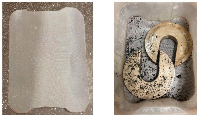
Figure 3. Crumb rubber pre-treatment with sodium hydroxide using a stainless-steel gauze.
