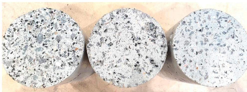
**Figure 6.** Different rubber content in cylinder specimens.
