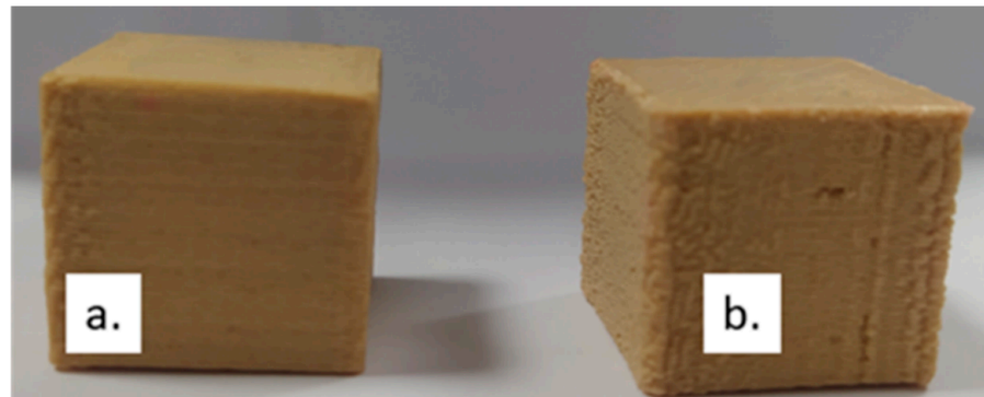
Figure 4. Experimental specimens manufactured with (a) SS = 110 mm/s, LH = 0.10 mm, and PT = 210 °C; (b) SS = 110 mm/s, LH = 0.25 mm, and PT = 200 °C.
