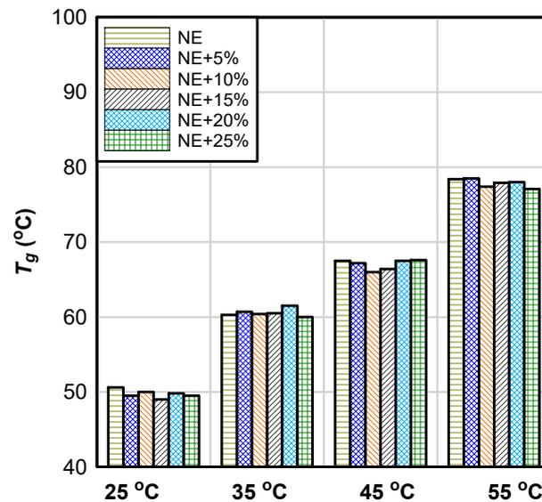
**Figure 7.** Glass transition temperature of neat and epoxy/CSR blends.
