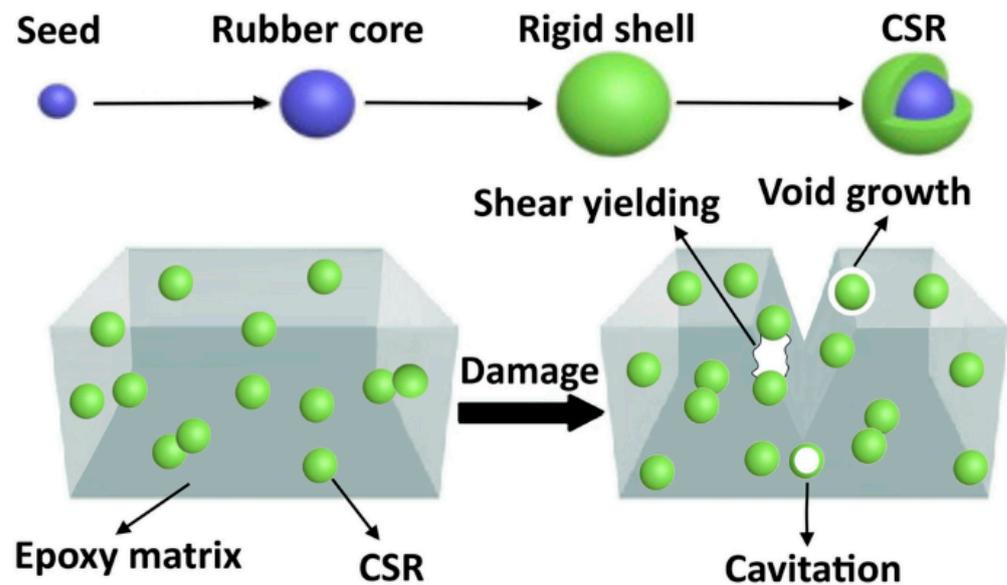
**Figure 1.** Toughening mechanism of CSR in epoxy matrix. (Reprinted with permission from Springer Nature Customer Service Centre GmbH: Springer, Journal of Materials Science, toughening of epoxy resin systems using core–shell rubber particles: a literature review by Mousavi et al. (2021) [29]).
