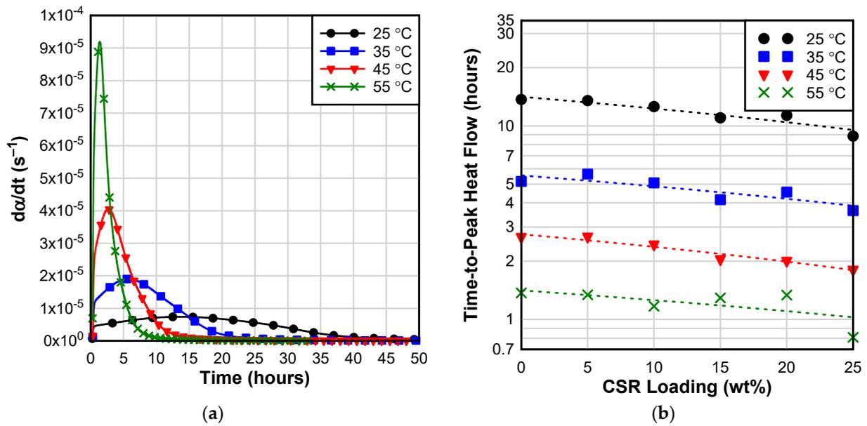
**Figure 3.** Isothermal calorimetry: (a) reaction rate of NE as a function of time and curing temperature; (b) effect of CSR loading on time-to-peak heat flow at different curing temperatures [dashed lines are only to guide eyes].
