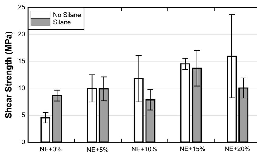
**Figure 10.** Single-lap shear test results: shear strength was computed by normalizing the maximum recorded load by the area of the adhesive joints.
