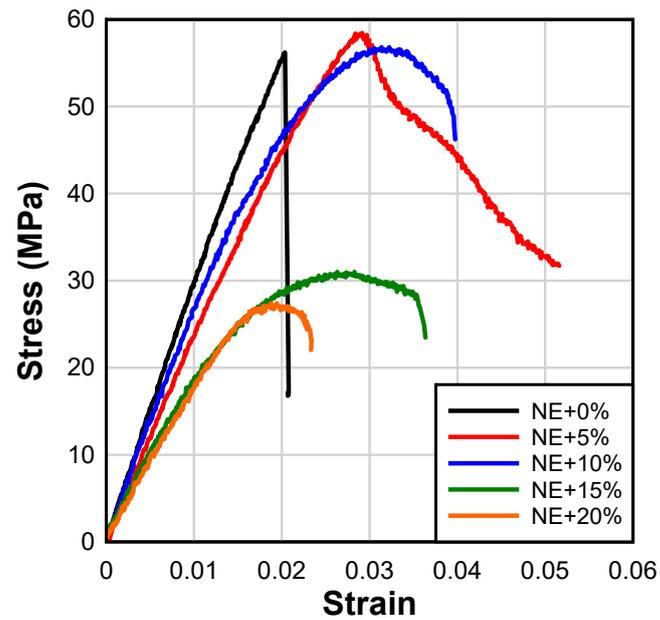
Figure 8. Typical stress–strain curves of adhesives.
