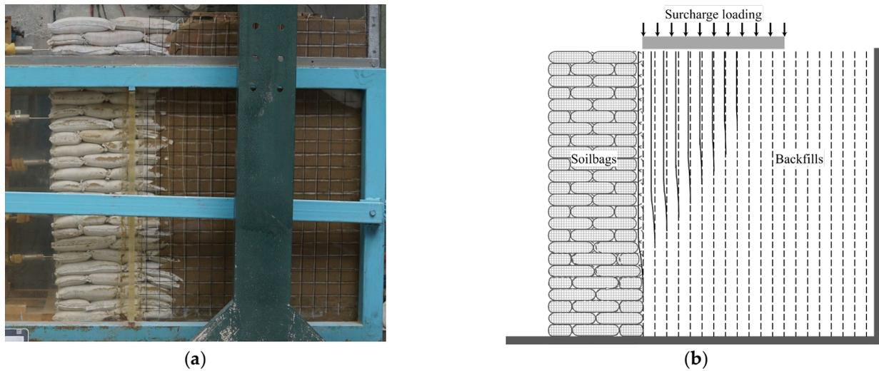
**Figure 2.** Deformation of the backfill in the wall subjected to surcharge stress of 4 kPa (a) photo; (b) schematic diagram.
