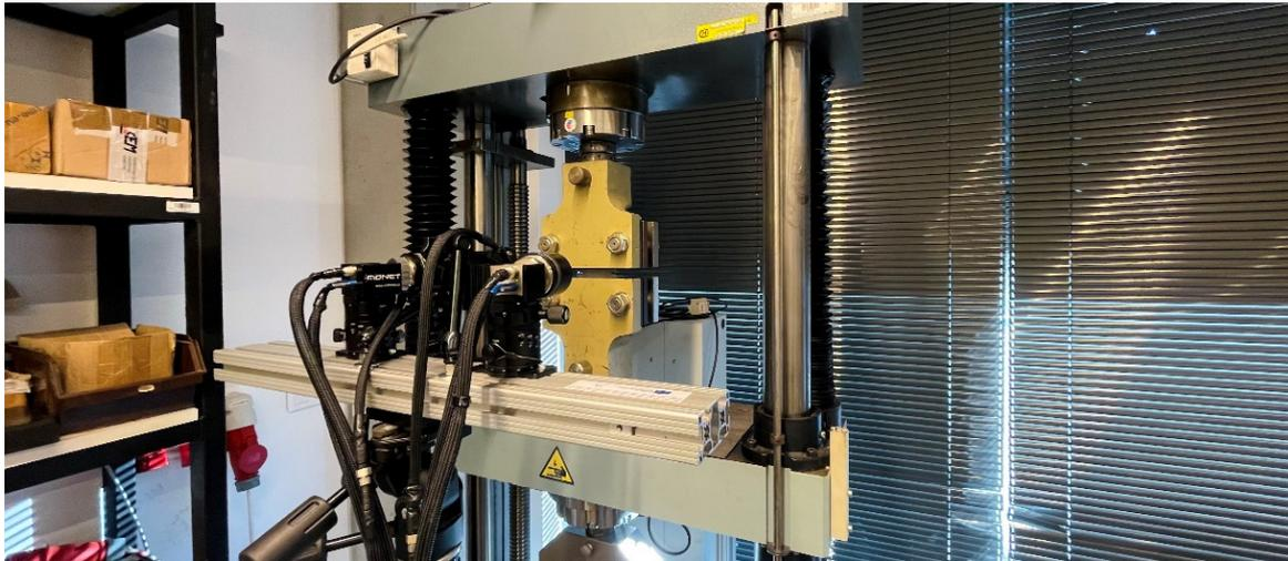
Figure 17. Realisation of the plane strain test on a TIRA Test 2300 testing device.
