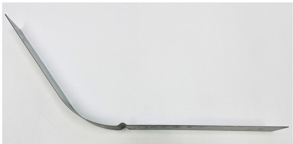
**Figure 25.** Specimen (real stamping) prepared by the strip drawing over the draw-bead.
