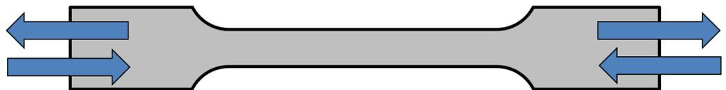
Figure 22. Schematic diagram of the specimen loading during the cyclic test.
