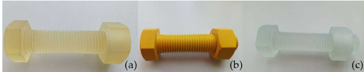
Figure 9. Screws and nuts are produced using the following techniques: (a) PolyJet, (b) FDM, and (c) SLA.
