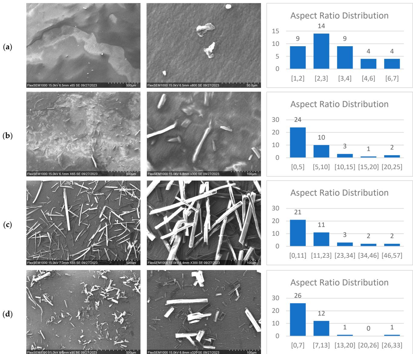
**Figure 1.** (a) SEM images and aspect ratio distribution of CNC using sulfuric acid, (b) SEM images and aspect ratio distribution of CMF using sulfuric acid, (c) SEM images and aspect ratio distribution of CMF using citric acid, (d) SEM images and aspect ratio distribution of CMF using oxalic acid.
