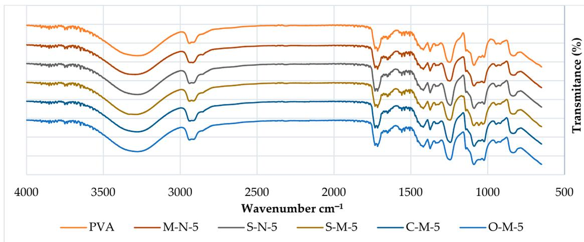
Figure 5. FTIR spectra of PVA cast films with 5% filler.
