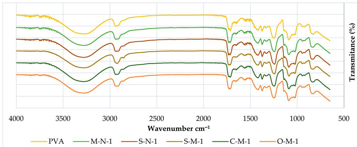
Figure 4. FTIR spectra of PVA cast films with 1% filler.
