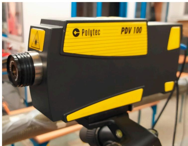
**Figure 8.** Laser for measuring (vibration speed).
