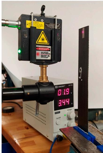
**Figure 7.** Laser for measuring (vibration displacement).
