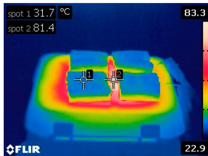
**Figure 5.** Experimental setup for monitoring phase change material leaks during operation.
