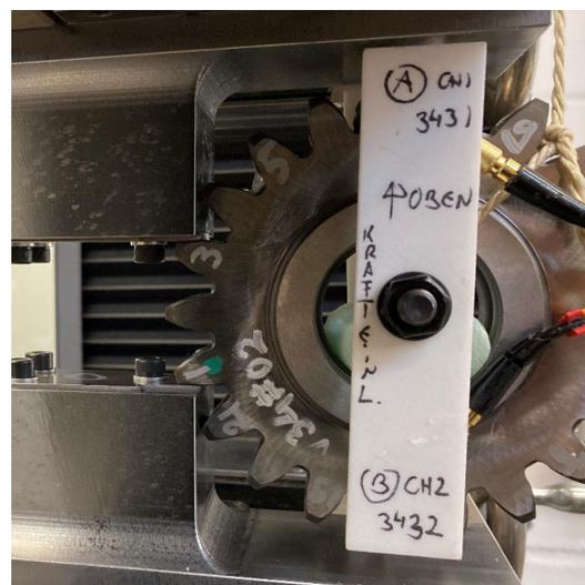
**Figure 10.** Experimental setup of the pulsator test.
