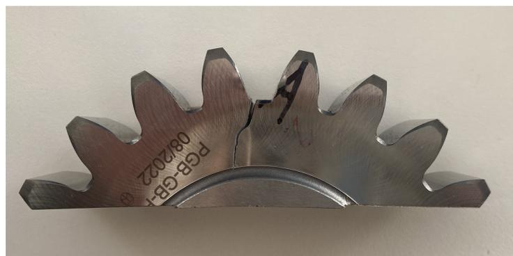
**Figure A1.** Crack propagation when indenting fragment C4 into the tooth gap (Test 2, front).
