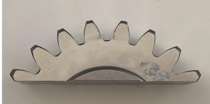
**Figure A4.** Crack propagation when indenting fragment C4 into the tooth gap (Test 3, back).
