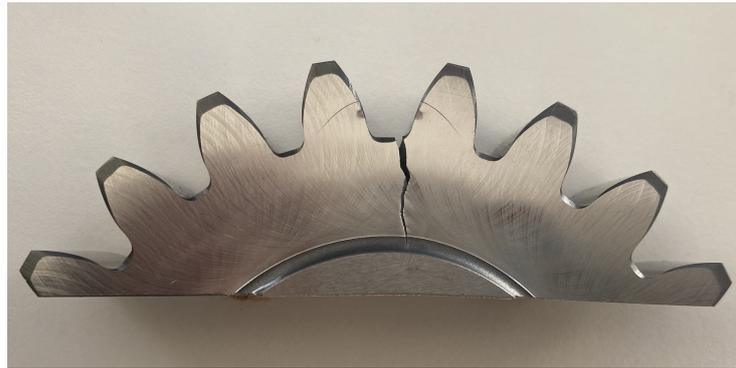
**Figure A2.** Crack propagation when indenting fragment C4 into the tooth gap (Test 2, back).
