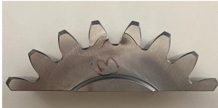
**Figure A3.** Crack propagation when indenting fragment C4 into the tooth gap (Test 3, front).
