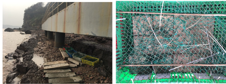
Figure 3. Sample preparation cured in a marine tidal environment.
