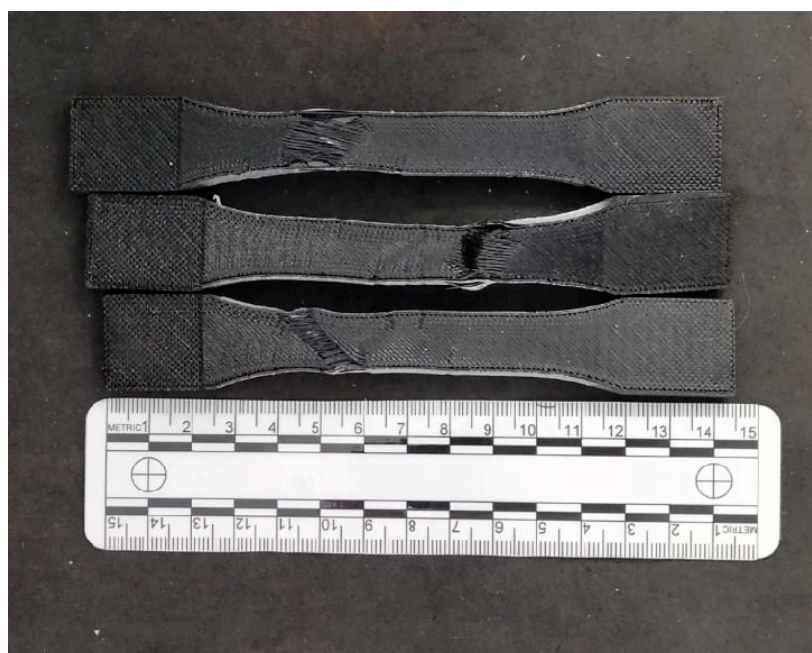
Figure 11. Samples after static tensile testing made of carbon fiber PET-G.
