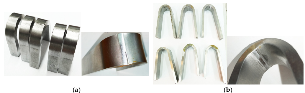
Figure 5. Example photos of specimens after the bending test: (a) TIG joint (2 T); (b) laser joints 3 L, 4 L in 16Mo3 steel.
