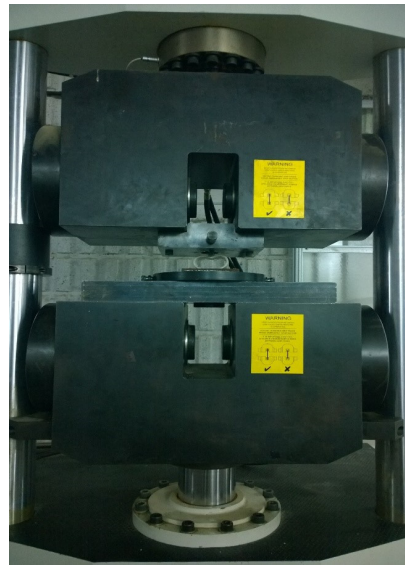
Figure 2. Setup for lateral indentation test of composite specimen B-04.
