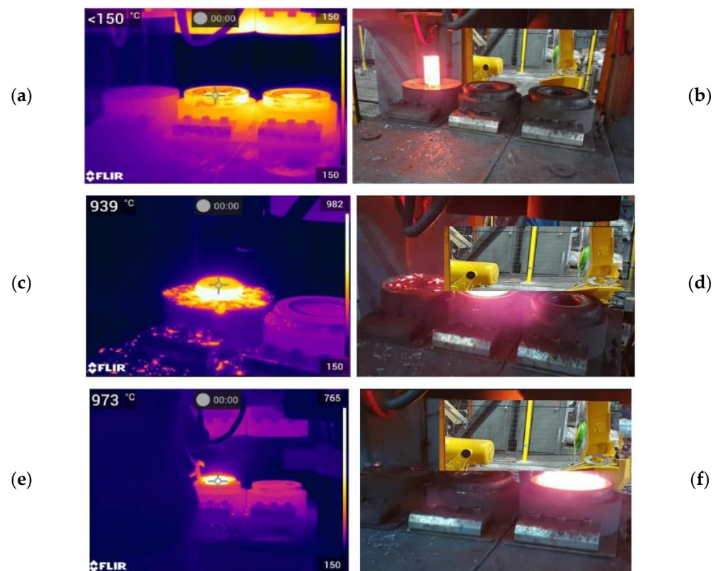
Figure 13. View of the consecutive operations realized on the crank press: (a) a thermogram with the heated tools, (b) a photograph of the heated charge placed on the lower tool for upsetting, (c) a thermogram of the deformed forging after upsetting, (d) the forging replaced by the robot to the roughing operation, (e) a thermogram after the roughing operation, and (f) the forging after the finishing forging operation.
