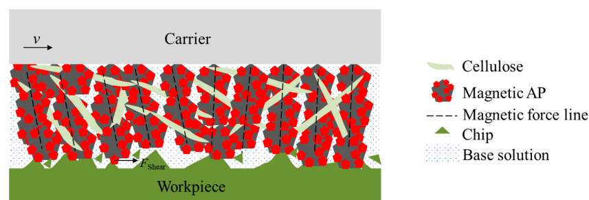
Figure 2. Schematic diagram of the magnetic abrasive particle polishing method.
