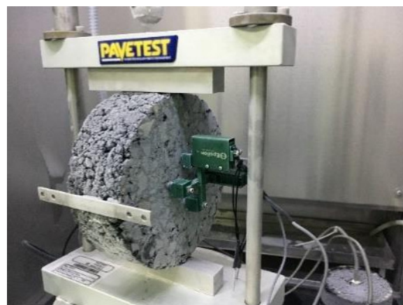
Figure 2. Test setup for IDT creep and strength tests.
