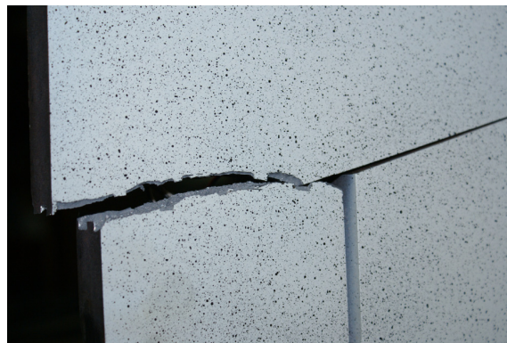
Figure 2. An example of a stochastic pattern applied to the elements of the tested railway joint.
