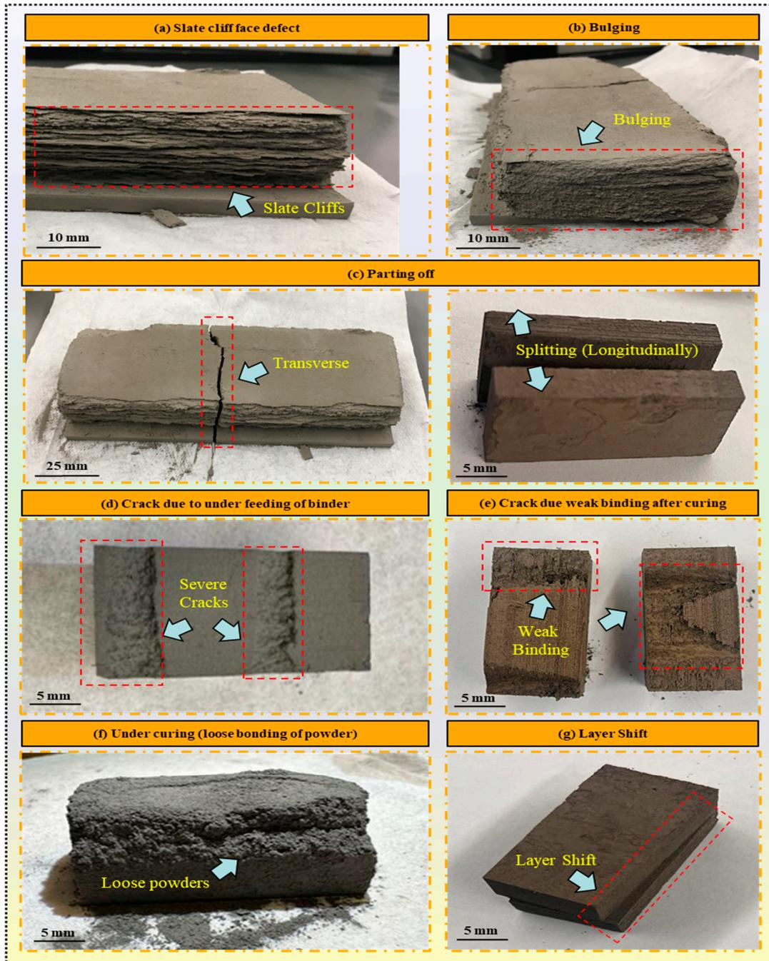
**Figure 9.** Illustration of mechanical defects observed post curing: (a) slate cliff face defect, (b) bulging, (c) parting off, (d) crack due to under-feeding, (e) crack due to weak binding, (f) loose bonding of the powder particles, and (g) layer shift.
