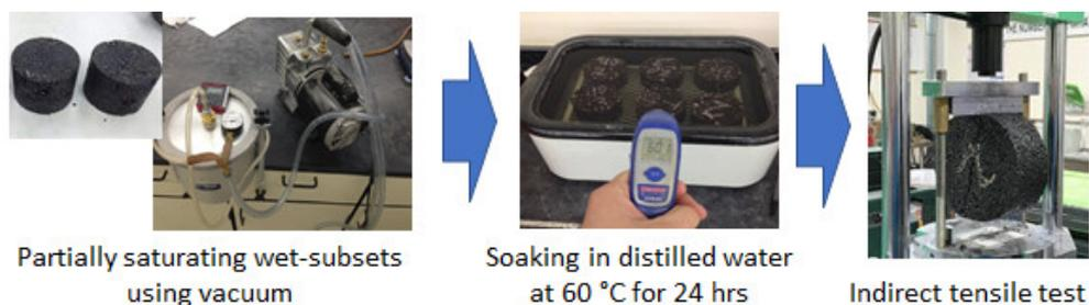
**Figure 6.** The procedure of the moisture susceptibility test.
